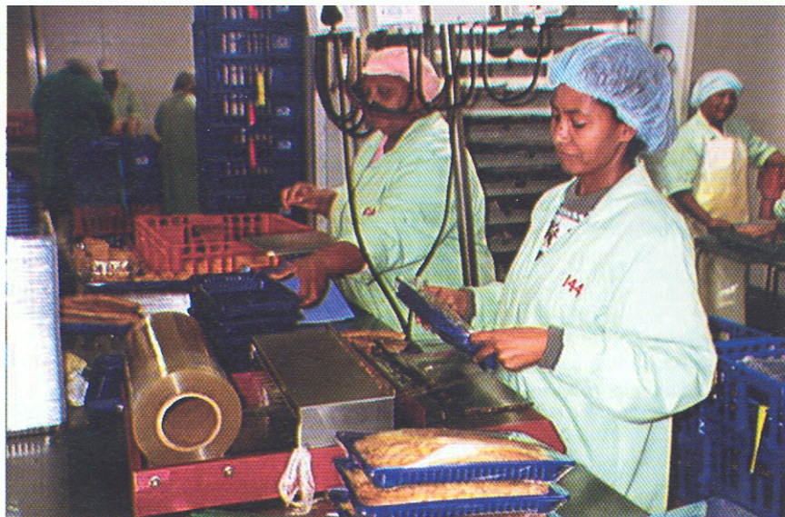
Photo 1. The heating of plastic wrapping during the packaging of fish products generates pyrolysis products that can cause asthma.
