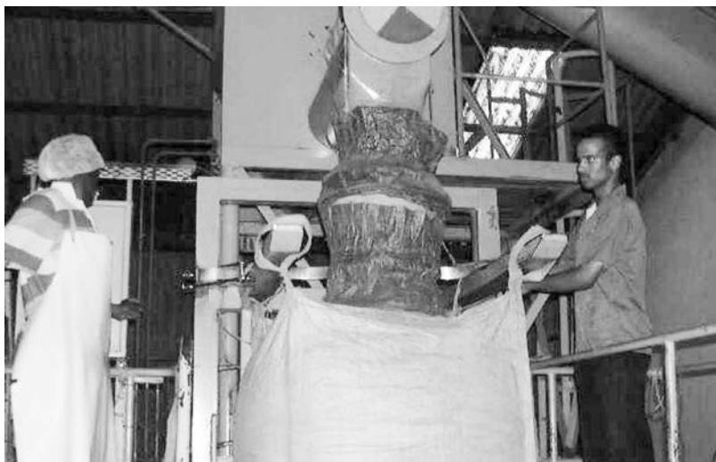
Figure 6.10. The introduction of a bagging operation in a fishmeal production plant operating with a chute and local exhaust ventilation can reduce dry bioaerosol emissions.
