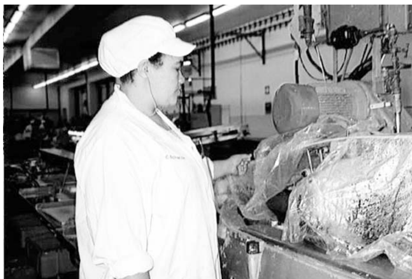
Figure 6.9. Bioaerosol emissions from the fish degutting machine can be reduced by enclosing the machine with a simple shroud of clear polythene.
