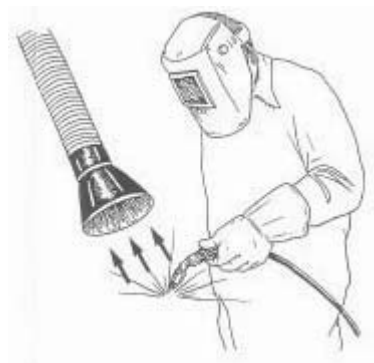
Figure 5.4.1. Gas-shielded welding with mobile local exhaust ventilation.
