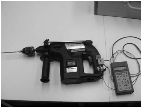
Figure 4.5.3. Vibration measurement from the handle of a drill. The figure illustrates the insertion of acceleration sensor to the handle of a drill. A three axial acceleration sensor can be fixed in a handle by tightly screwing or gluing so that the drill can be used for practical work.
