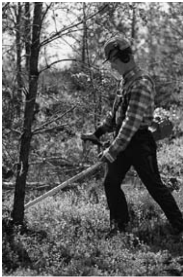
Figure 4.5.6. Forestry clearing saw in action. The manufacturer notifies purchasers that the equivalent vibration acceleration is less than 5 \text{ m/s}^2 , a level that will not exceed limit values.
