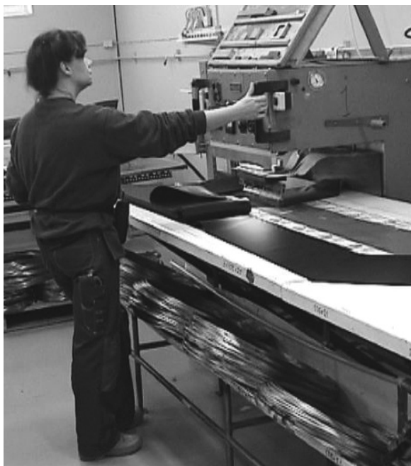
Figure 4.6.3. Radiofrequency plastic sealer used in the tarpaulin industry. The operator gets high whole body exposure, and the hands are highly exposed. It would be desirable for the machine to be operated by remote control so that the worker could step back from the machine. A substantial RF current can also flow into the body of the operator depending on the material in the floor – i.e. how much RF ground the floor is.
