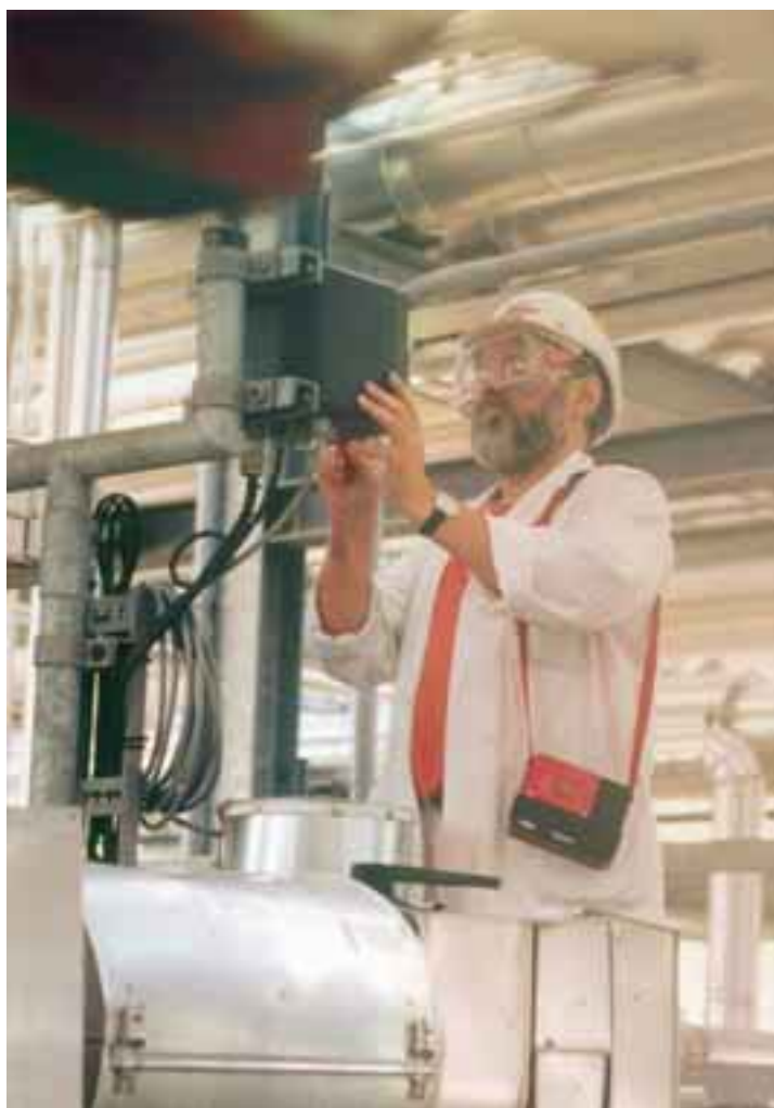
MULTIWARN enables continuous measurements of airborne contaminants (e.g. carbon dioxide, oxygen, carbon monoxide, hydrogen sulphide and hydrocarbons) at workplaces. Copyright Draeger Safety AG & Co.KGaA, Luebeck, Germany
