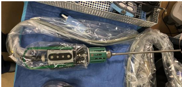
Figure 6: Zero-degree robotic endoscope with sterile draping
