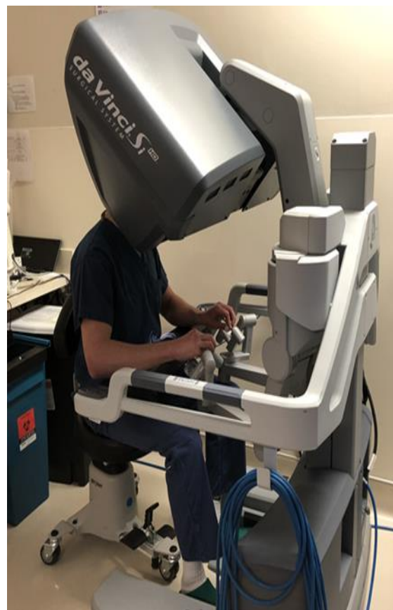
Figure 1. Surgeon sits at a separate console and directs movements of the robotic arms and surgical instruments
