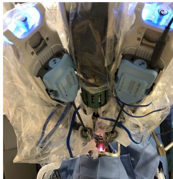
Figures 3 b,c: Patient Cart: Surgical robot appears with sterile draping and three surgical arms are seen entering into the oral cavity (centrally-positioned surgical endoscope with adjacent instrumented arms)
