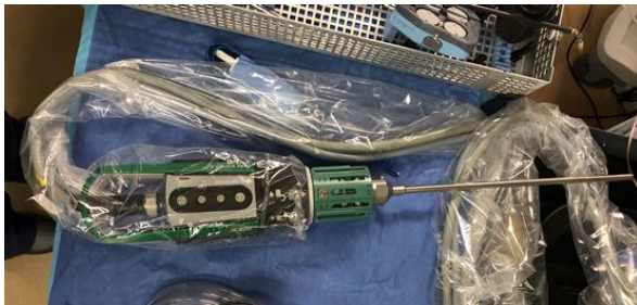
Figure 6: Zero-degree robotic endoscope with sterile draping
