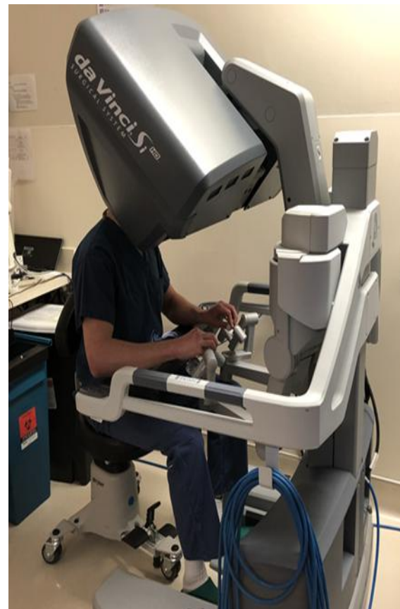
Figure 1. Surgeon sits at a separate console and directs movements of the robotic arms and surgical instruments
