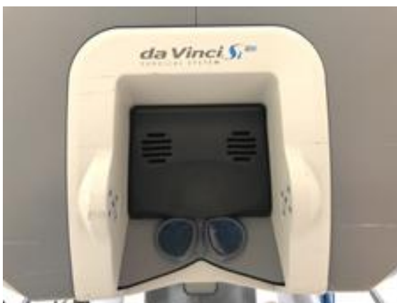
Figure 2d: Stereo Viewer
