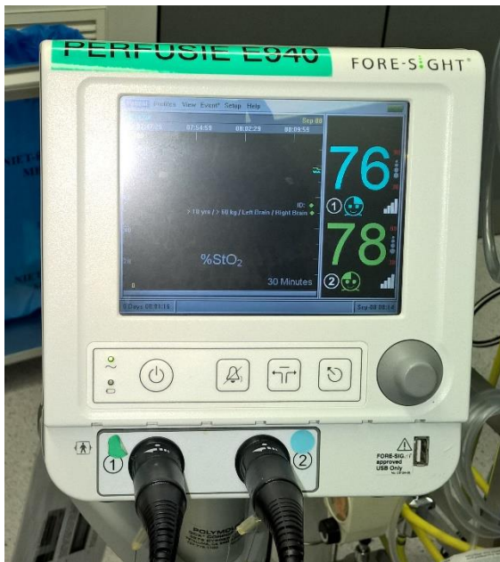
Figure 11b: Symmetry of oxygenation can be followed throughout the procedure using the ForeSight system ®
