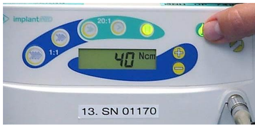
Figure 33: Drill setting for inserting the fixture
