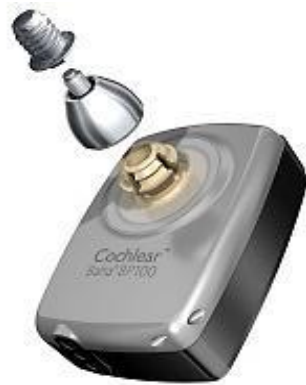
Figure 3a: Cochlear osseointegration system with coupling inside the abutment
