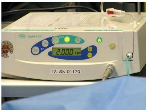
Figure 28: Drill setting for initial drill holes
