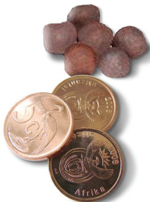
Processed iron ore pellets used in the steel making industry, with an RSA 5c coin, shown to scale
