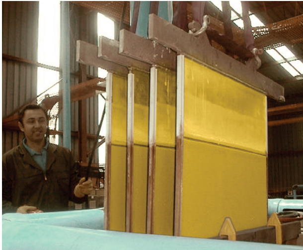
Steel cathode plates with gold plated on them
