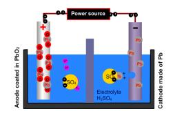
power source, e.g. another battery. The lead electrode must be connected to the [positive/**negative**] terminal of this other battery. This pulls electrons from the [lead/lead dioxide] electrode and forces electrons into the [lead/lead dioxide] electrode. This causes the reactions which had occurred in the discharging reaction to take place [in the same direction/in reverse].
