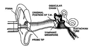
Figure 1: Tympanometer probe tip in the ear canal
