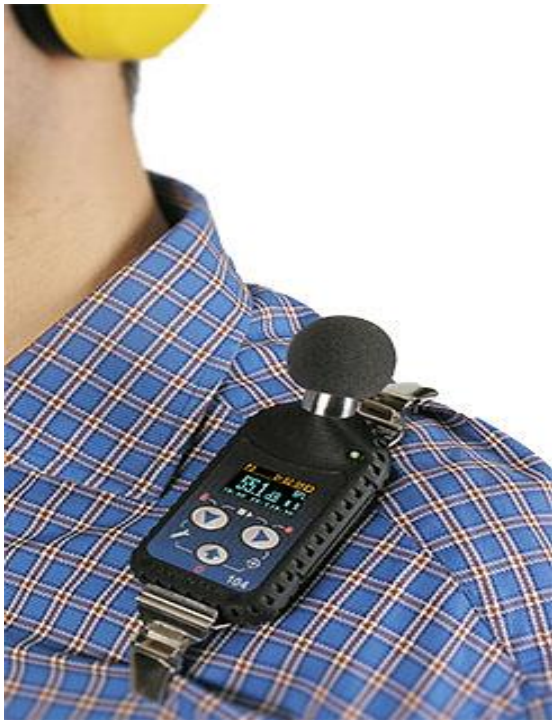
Figure 4: Noise dosimeter mounted on the shoulder
