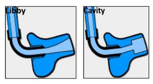
Figure 10: Libby Horn and Cavity modifications
