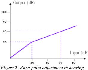
Figure 2: Knee-point adjustment to hearing aid
