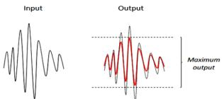
Figure 24: Automatic gain control
