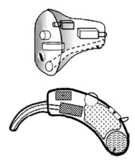
Figure 5: Custom-made and Behind-the-Ear (BTE) hearing aids
