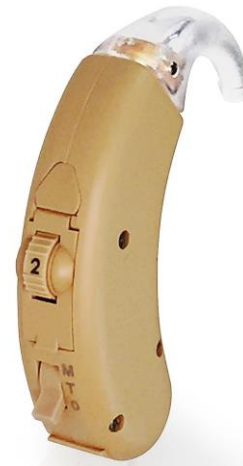
Figure 1: On-off switch and volume control wheel mounted on hearing aid case of analogue hearing aid
