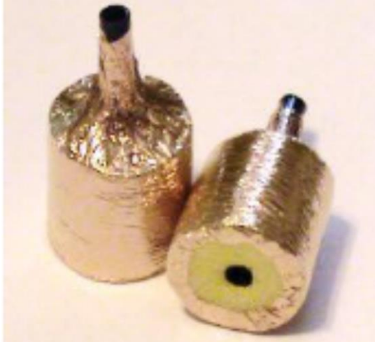
Figure 5: Example of tip-trode electrode
