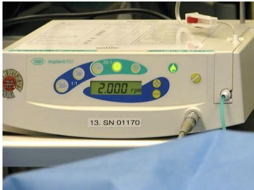
Figure 28: Drill setting for initial drill holes
